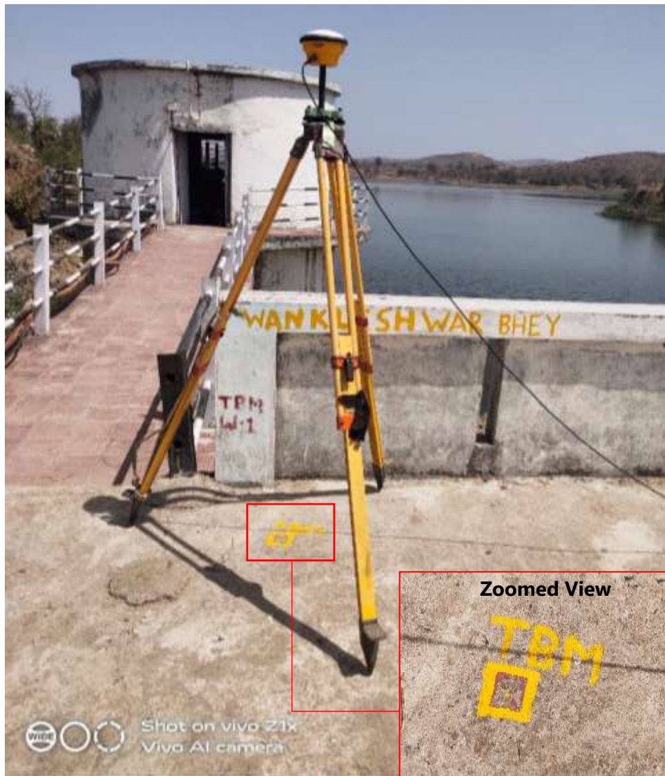
Figure 3.1: Wankleshwar Bhey Temporary Benchmark 1 (Wankleshwar Bhey TBM)
